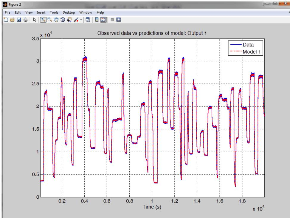
Figure 5. Observed and Predicted Output Data of the Model
