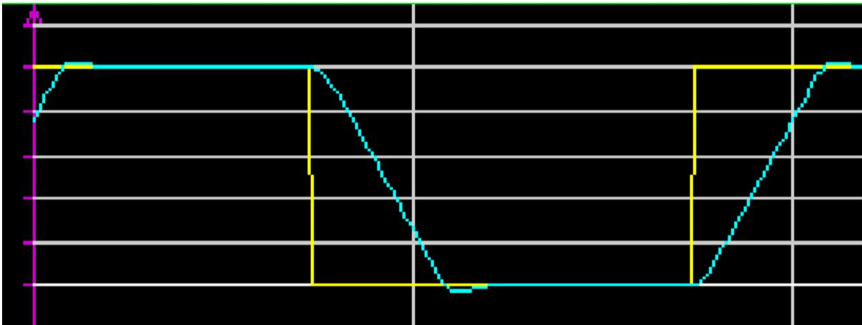
**Figure 10. Response of the DC Motor Position Proportional Controller.**
