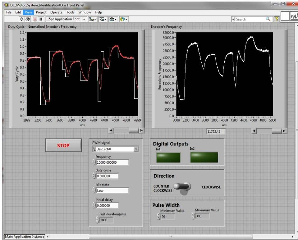
Figure 2. Front Panel of the LabVIEW vi.
