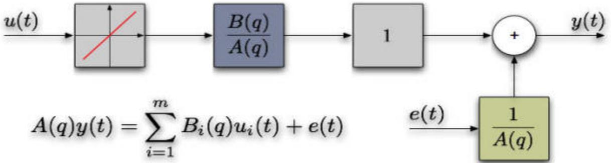
Figure 4. Autoregressive Exogenous (ARX) model's structure
