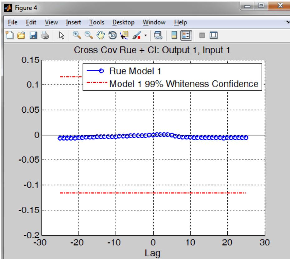
Figure 6. Cross-correlation between the Prediction Error and the Input
