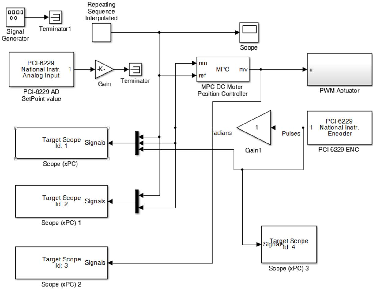
**Figure 9. DC Motor Position Control System using a Model Predictive Controller (MPC).**
