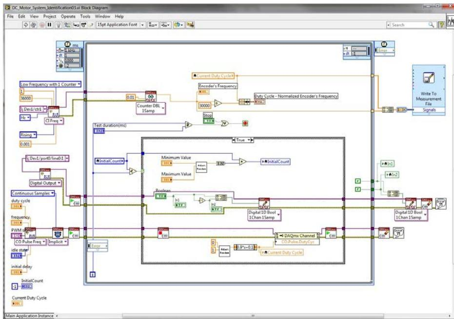
Figure 3. Block Diagram of the LabVIEW vi.
