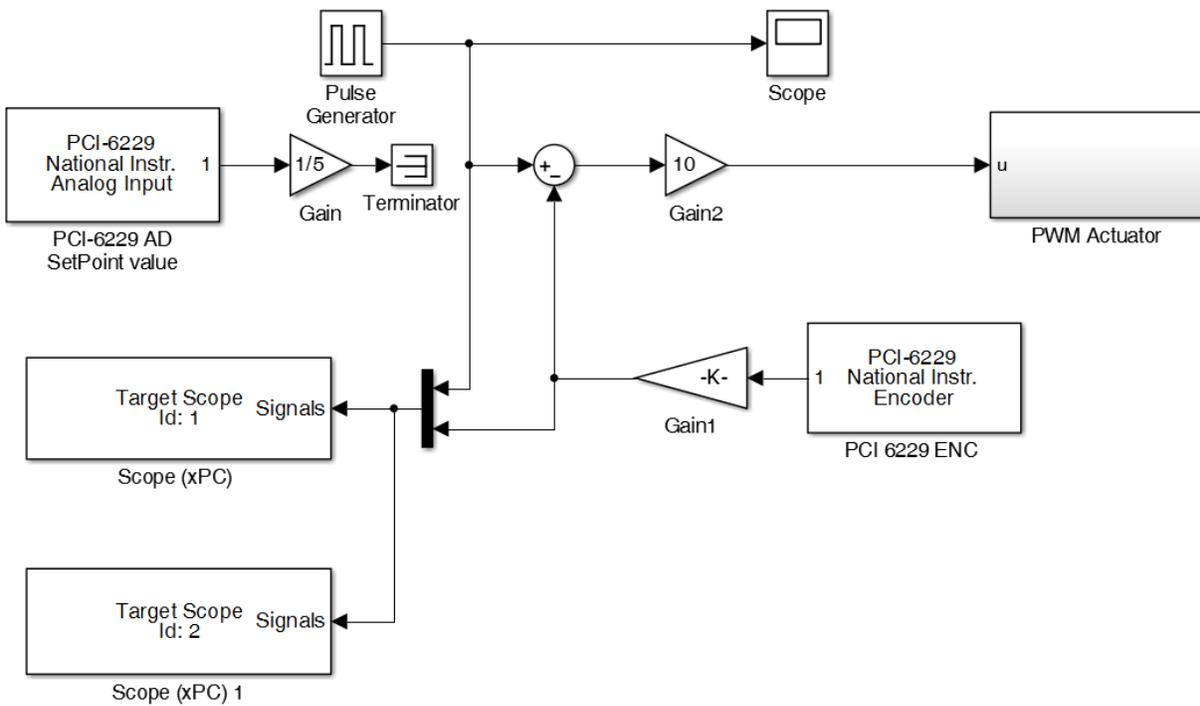
Figure 8. DC Motor Position Control System using a Proportional Controller.
