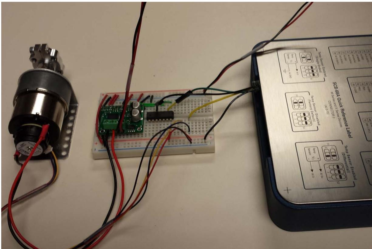
**Figure 1. Test Stand for DC Brushed Motors.**
